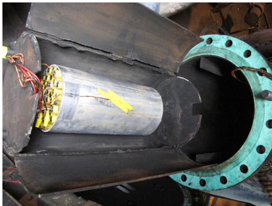
Fig. 14 — Pressurizable containment configuration
