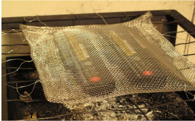
Figure 13 Laptop cells in their container placed on burner before test 7
