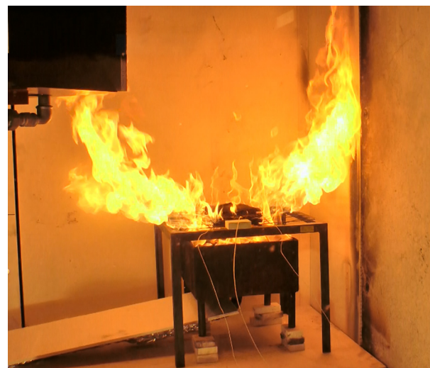
Fig. 6. Outbursts from EIG 100% SOC (test 1).
