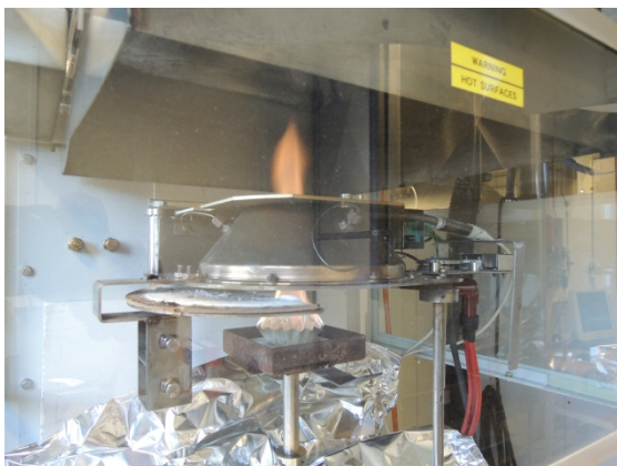
Figure 11. Open container placed underneath cone heater and ignited
