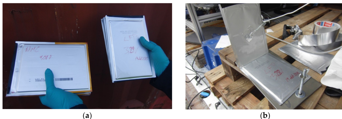
Figure 12. (a) Li-ion pouch cells used for the test. All NMC/LMO cells were charged to 4.1 V/cell and the LFP cells to 3.3 V/cell, respectively, before the test. (b) Stacks of 5 cells were clamped between metal plates with thermocouples placed between the bottom cell, nearest the heating plate, and the second cell in the stack.
