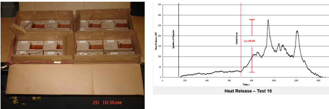
Fig. 10 — Bulk storage test, E type cells
