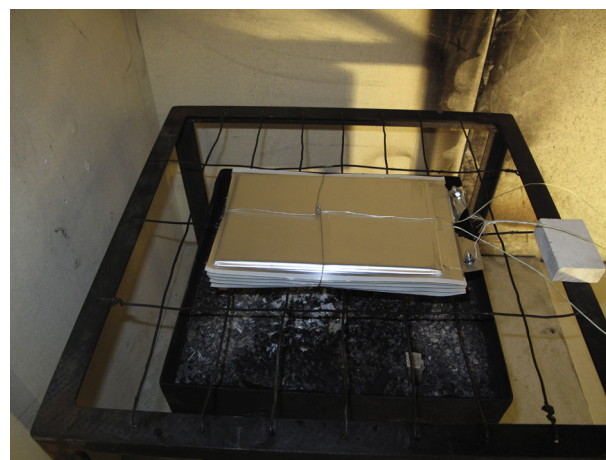
Fig. 2. The 5-cells pack of EiG cells placed on a wire grating.
