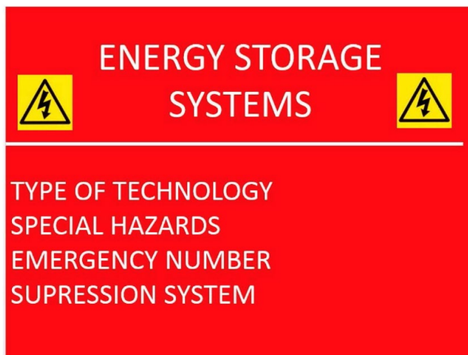
Figure B1 – Example of ESS Signage
