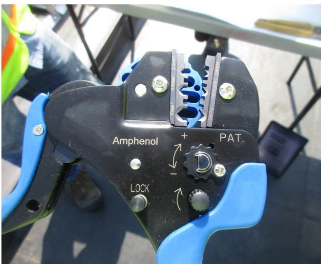
Figure 6. Crimping tool for one brand/type of connector.
