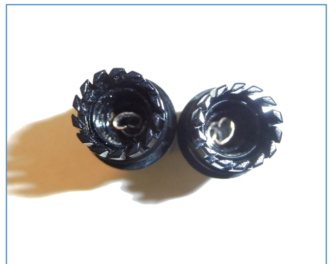
Figure 7. Conductors can pull out from poorly crimped parts.
